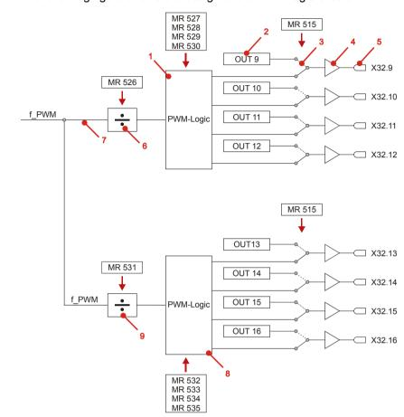
Principle of a PWM logic circuit The module JX3-DIO16 generates PWM signals in an internal logic circuit. The following figure shows the design of the PWM logic circuit:
