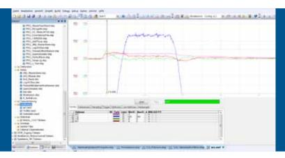
Oscilloscope mode is an integral feature of JetSym. The parameters and scaling are freely selectable; data can be saved in CSV format.
