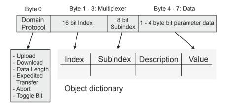
The 8 bytes of the SDO (as shown here) have been stored to the data range of the CAN message. The device is addressed by means of the SDO in the identifier
