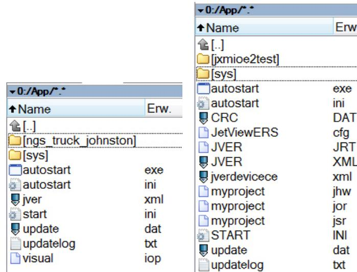
The screenshot to the left shows the file system of the old S platform. The visualization application is stored to an \*.iop file. In the given example it is the file **visual.iop**.
