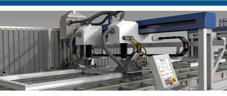
Cleaning machines machine and clean the window profiles after the welding process. For example, weld seams are removed and additional machining of posts and floating mullion casements is performed optionally. Hand-operated individual machines up to fully automatic CNC-controlled cleaning machines are in use here.
