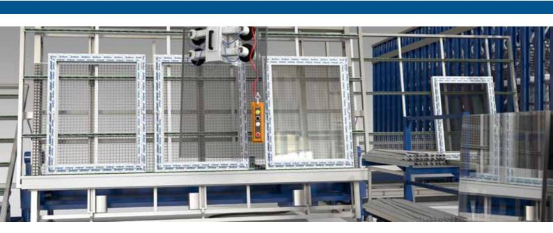
The logistical challenges for glass panels are especially high. Along with enormous transport weights and different formats, it must be possible to store and transport the material safely without any damage. Window and glass elements are then joined in an automated process.
