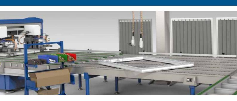
The essential tasks of automatic installation of fittings are drilling and bolting components of all kinds, e.g. fittings and reinforcements.
