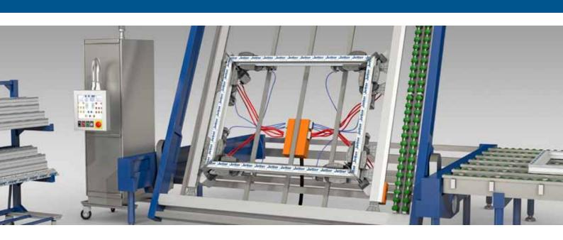
Plastic profiles are welded in a versatile way with up to eight welding heads in vertical or horizontal orientation. There are also many manual and fully automatic machining solutions available for this production step.
