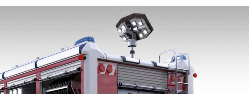
Proper illumination in the vehicle or around it, as well as of the scene of emergency is based on a sophisticated control concept taking into account the different requirements placed on the lighting systems used. Exact direction of light masts and lighting heads through coordination of motors and mechanics is among the primary tasks of the applied controller. The integrated controllers by Jetter AG are able to cover the respective functional requirements.
