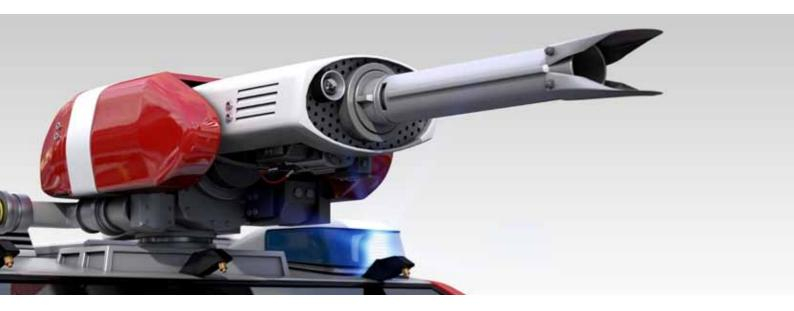
With flow rates of 1,000 l/m up to 4,000 l/m and throwing ranges up to 90 m, monitors are particularly apt for fighting fires with large amounts of water from great distances. Besides a continuous flow of water, exact direction of monitors to the object is crucial. For coordinating the involved functions, Jetter uses an especially designed controller which can be customized if need be.
